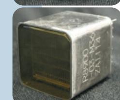
▲ Photomultipliers The PMT surface has 85% active area, having 6 × 6 pixels with a total area of 26.2 mm square.
